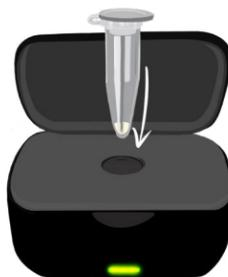
**2b** Place the Assay Tube in the Instrument. Open the Assay Tube lid.
